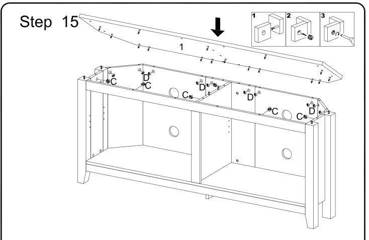
Carefully attach panel (1) to the assembly using cam bolts and dowels as guides. Insert cam locks (C,D) into the assembly as shown above and tighten with a screwdriver.
