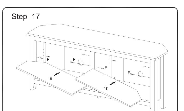
Insert shelf support pins (F) into the assembly at desired shelf heights. Carefully place shelves (9,10) on shelf support pins (F).
