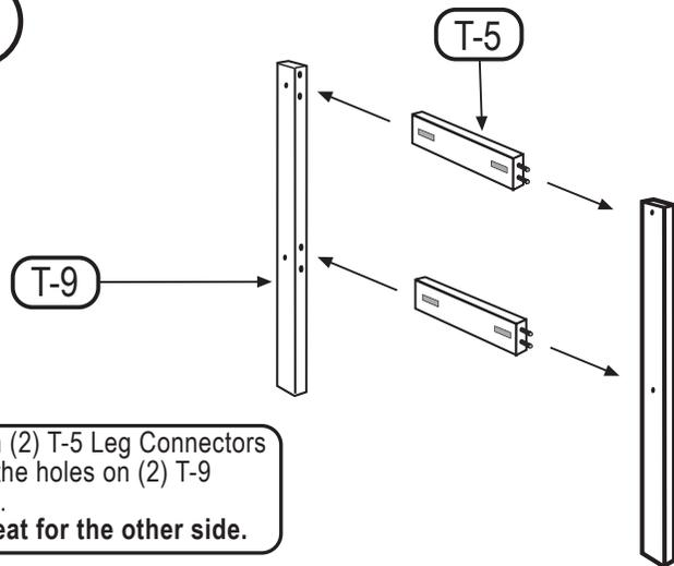
Push (2) T-5 Leg Connectors into the holes on (2) T-9 Legs.
