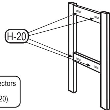
Secure the Leg Connectors to the Legs using (4) Wood Screws (H-20).
