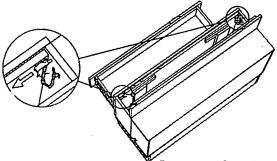
Remove Safety Chain (When Closing Secure Safety Chain) Start To Open 1st Deck
