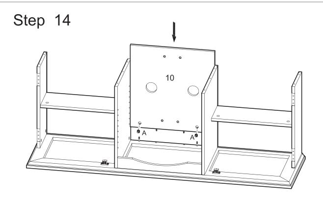
Carefully slide back panel (10) into place along the back of the stand assembly. Use cam bolts and dowels as guides. Insert cam locks (A) into back panel (10) and tighten with a screwdriver.
