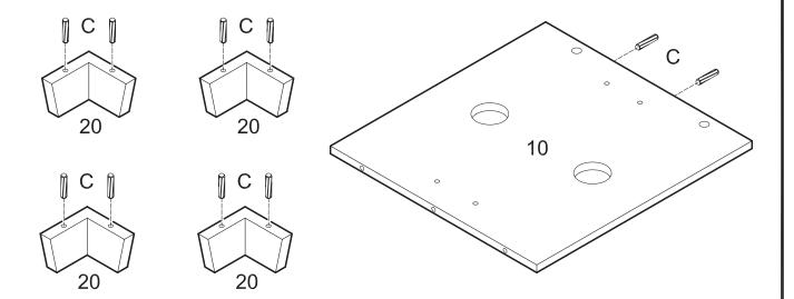
Insert dowels (C) into feet (20) and back panel (10).
