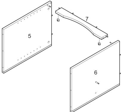
Insert cam locks (A) into slat (7). Attach panels (5,6) to slat (7) using cam bolts and dowels as guides. Tighten cam locks (A) with a screwdriver.
