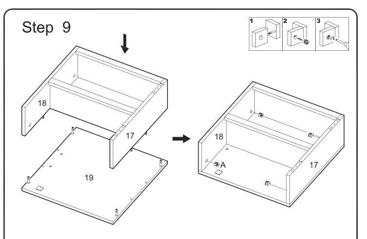
Attach the panel assembly (17,18) to door (19) using cam bolts and dowels as guides. Insert cam locks (A) into panels (17,18) and tighten with a screwdriver.
