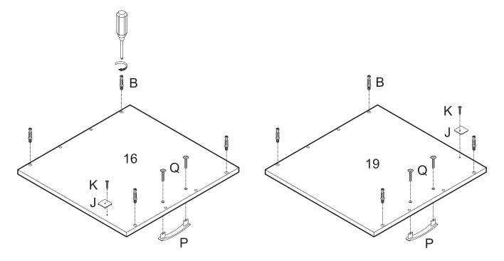
Screw cam bolts (B) into doors (16,19). Attach door stopper plates (J) to doors (16,19) using screws (K). Attach handles (P) to doors (16,19) using bolts (Q).
