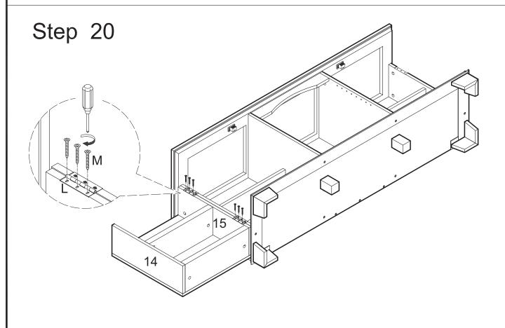
Attach door assembly (14,15) to the stand assembly at door hinges (L) using screws (M).
