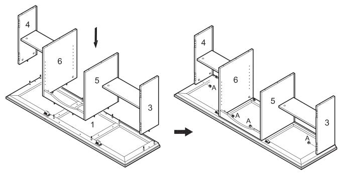
Attach the panel assembly from the previous step to stand top (1) using cam bolts and dowels as guides. Insert cam locks (A) into panels (3,4,5,6) and tighten with a screwdriver. *Note that two cam locks (A) will be inserted into each panel (3,4,5,6)*.
