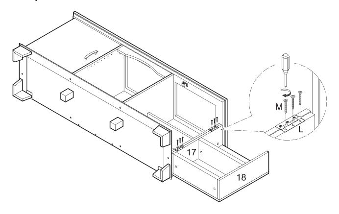
Attach door assembly (17,18) to the opposite side of the stand assembly at door hinges (L) using screws (M).
