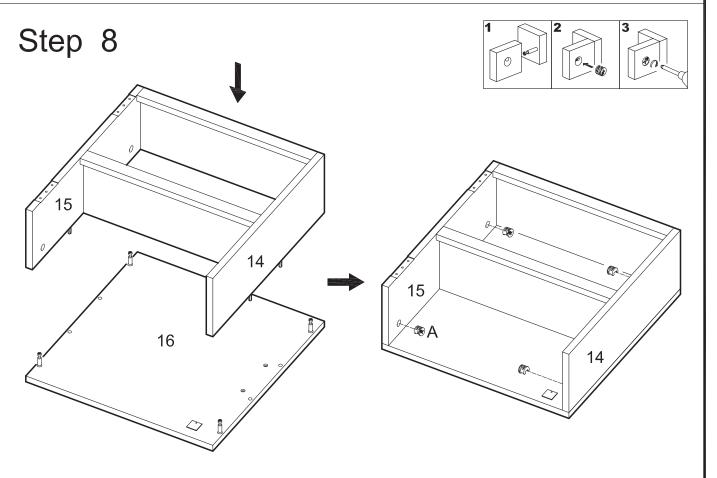
Attach the panel assembly (14,15) to door (16) using cam bolts and dowels as guides. Insert cam locks (A) into panels (14,15) and tighten with a screwdriver.
