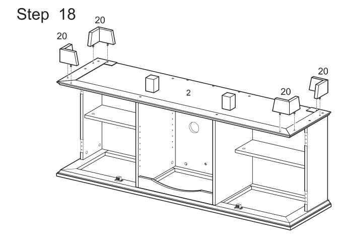
Attach feet (20) to stand base (2) using dowels as guides.
