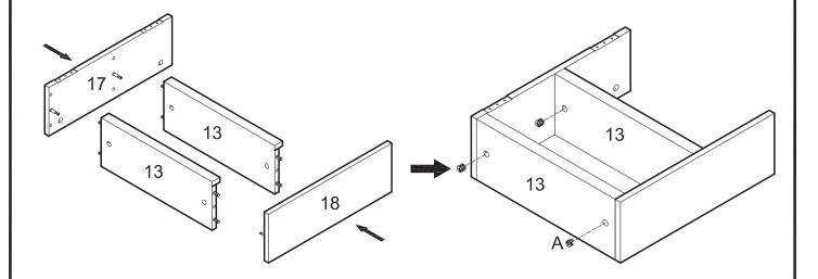
Attach panels (17,18) to the second set of shelves (13) using cam bolts and dowels as guides. Insert cam locks (A) into shelves (13) and tighten with a screwdriver. *Note that two cam locks (A) will be inserted into each shelf (13)*.
