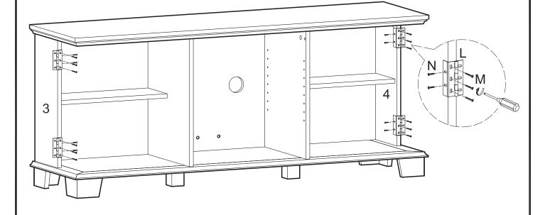
Attach door hinges (L) to panels (3,4) using screws (M,N).
