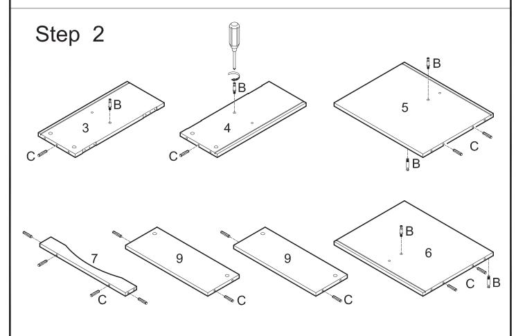
Screw cam bolts (B) into panels (3,4,5,6). *Note that one cam bolt (A) will be screwed into each side of panels (5,6).* Insert dowels (C) into panels (3,4,5,6), slat (7) and shelves (9).
