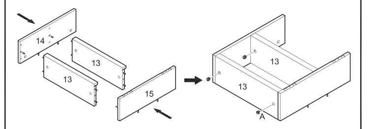
Attach panels (14,15) to shelves (13) using cam bolts and dowels as guides. Insert cam locks (A) into shelves (13) and tighten with a screwdriver. *Note that two cam locks (A) will be inserted into each shelf (13)*.
