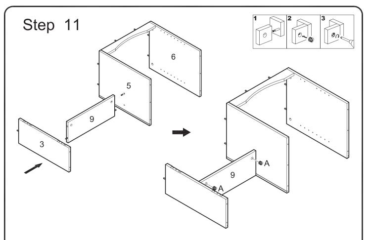
Attach shelf (9) to panel (5), then panel (3) to shelf (9) using cam bolts and dowels as guides. Insert cam locks (A) into shelf (9) and tighten with a screwdriver.
