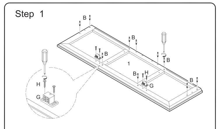
Screw cam bolts (B) into stand top (1). Attach door stoppers (G) to stand top (1) using screws (H).
