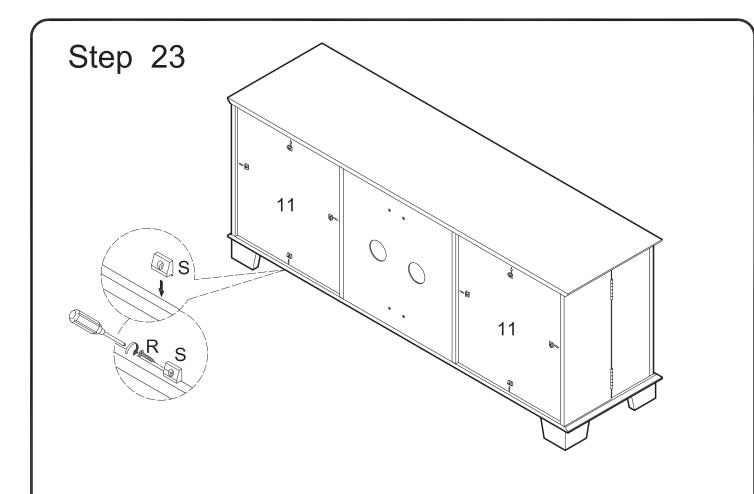
Secure back panels (11) using plastic wedges (S) and screws (R).
