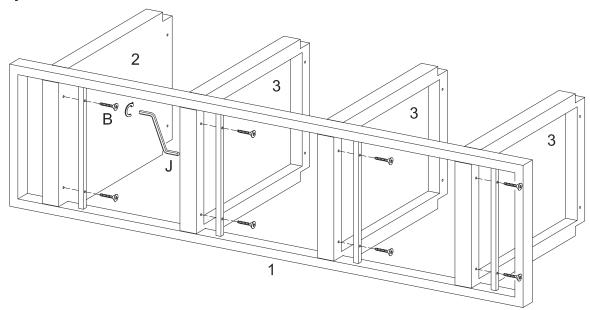
Place the Metal  $\,$  Side Panel  $\,$  (1) Horizontially , assamble the Shelf  $\,$  (2) for the top and Shelf  $\,$  (3) after by using Screw  $\,$  (B) and the Wrench  $\,$  (J)
