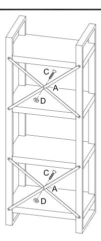
To ensure the sercurity for the Cross Bar (A), please put Screw (C) and Nut (D) to secure it
