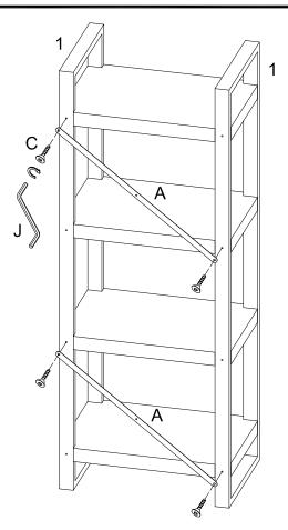
Stand up the Shelf and Secure the Cross Bar (A) at the back by using Screw (C) and Wrench (J) for one side.
