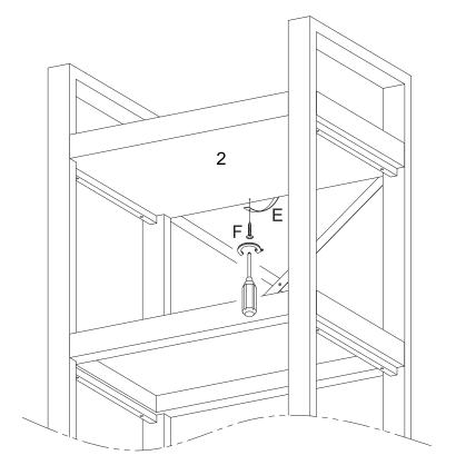
Attach the other End of the Cloth Belt (E) under the bottom of Panel (2) by Screw (F) and Screw driver
