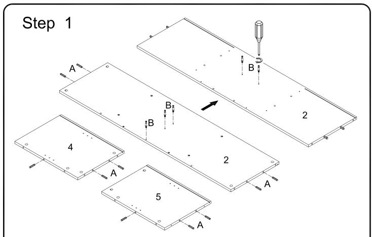
Insert the Wooden Dowel (A) to the Bottom Panel (2) and Side Panel (4)(5). Insert the Cam Bolt (B) to the Bottom Panel (2) for both sides.
