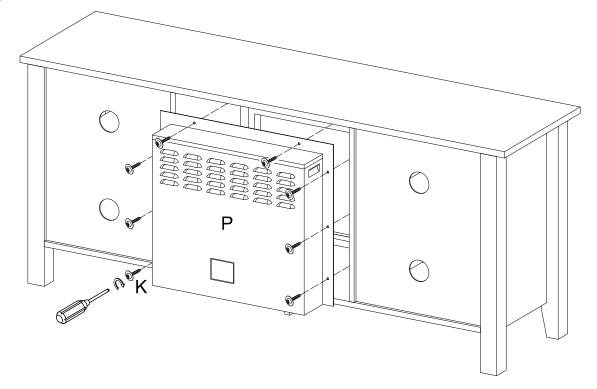
Assemble the Fireplace Insert (P) to the Stand and secure it with Screw (K)
