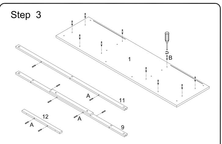
Insert the Cam Bolt (B) to the Top Panel (1), Insert the Wooden Dowel (A) to the Front Panel (9,11,12)
