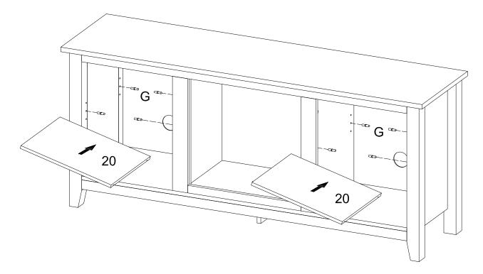
Input the Shelf Support Pin (G) to the Stand and place the Wooden Shelf (20) on top
