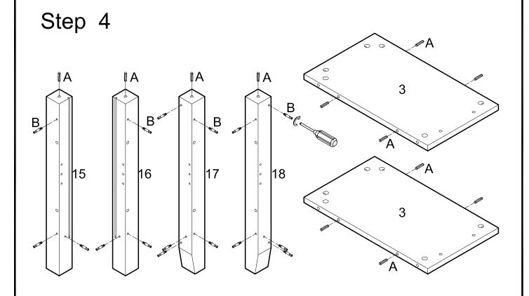
Insert the Wooden Dowel (A), Cam Bolt (B) to the Wooden Legs (15,16,17,18) Insert the Wooden Dowel (A) to the Side Panel (3)
