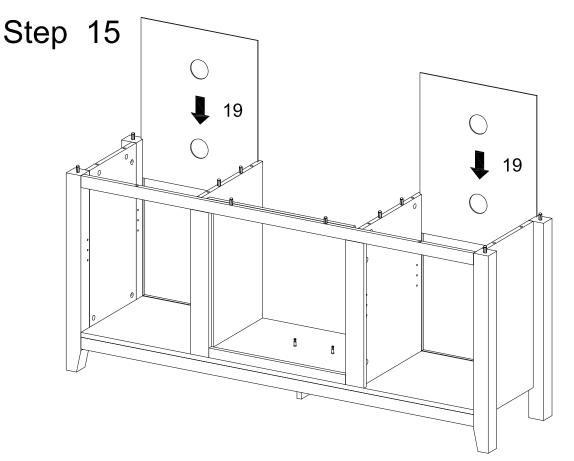
Right Up the Stand and slot in the Back Panel (19) to the Side Panels
