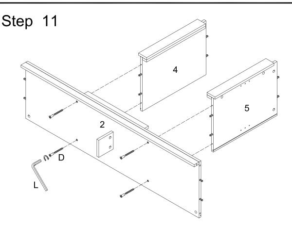
Assemble the Side Panel (4,5) to the Bottom Panel (2) and secure it by Bolt (D) and Wrench (L)
