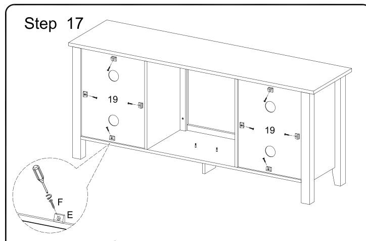
Use Flat-Head Screw (F) and Plastic Wedge (J) to secure the Back Panel (19)
