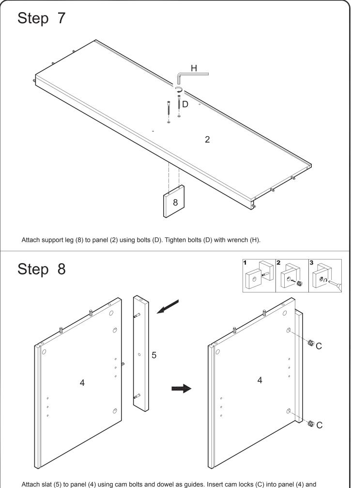
tighten with a screwdriver.
