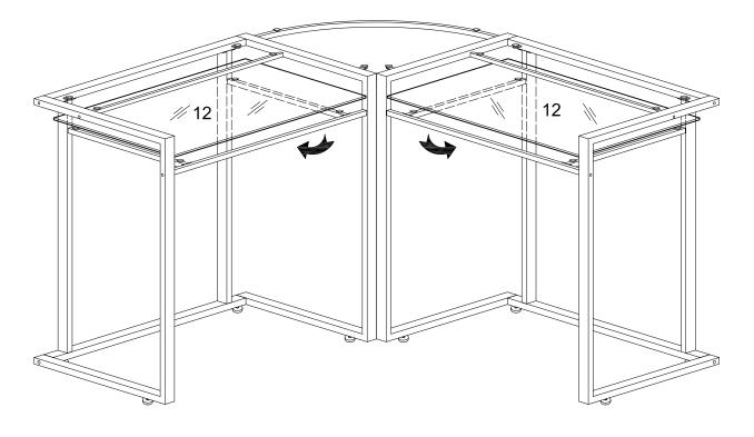
Carefully lay glass (12) into place and gently press on the suction cups to secure.
