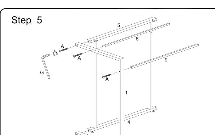
Attach lower crossbar (4), upper crossbar (5) and support bars (6,9) to leg (1) using long bolts (A). Tighten long bolts (A) with wrench (G).
