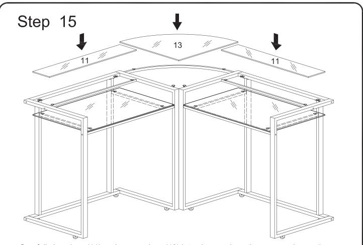
Carefully lay glass (11) and corner glass (13) into place and gently press on the suction cups to secure.
