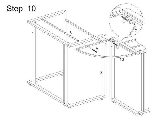
Attach leg (3) and crossbar (6) to corner frame (10) using long bolt (A) and bolt (C). tTighten all bolts with wrench (G).
