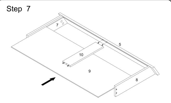
Carefully slide drawer panel (9) using the thin grooves. Insert support bar (10) into drawer panel (5).
