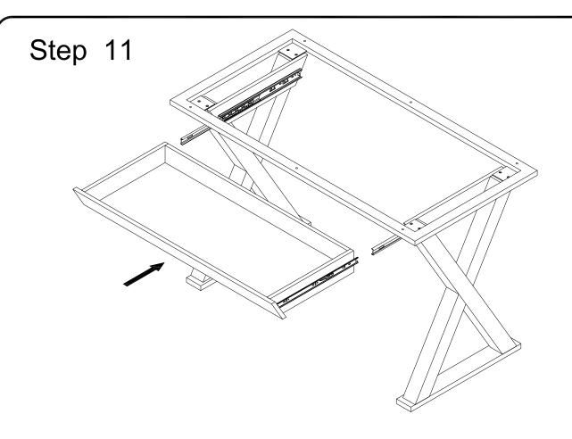
Carefully insert drawer assembly to assembled unit.
