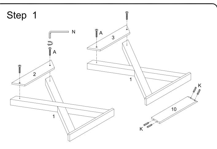
Attach side panels (2,3) to legs (1) using bolts (A). Insert wooden dowels (K) to support bar (10).
