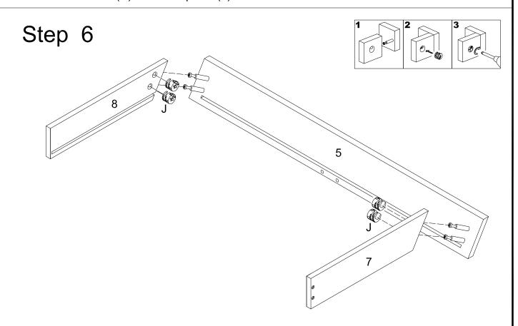
Attach drawer panel (5) to drawer panels (7,8) using cam locks (J).
