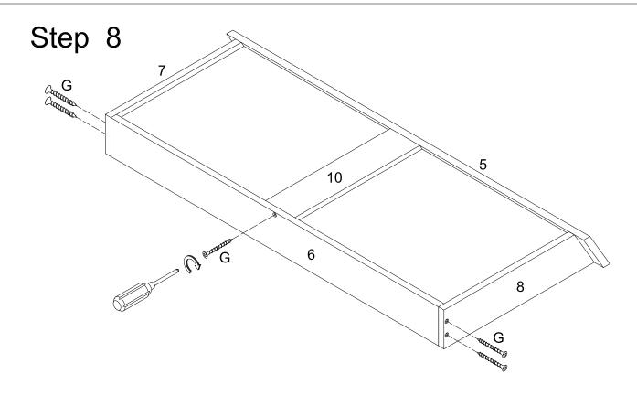
Attach drawer panel (6) to panels (7,8,10) using screws (G).
