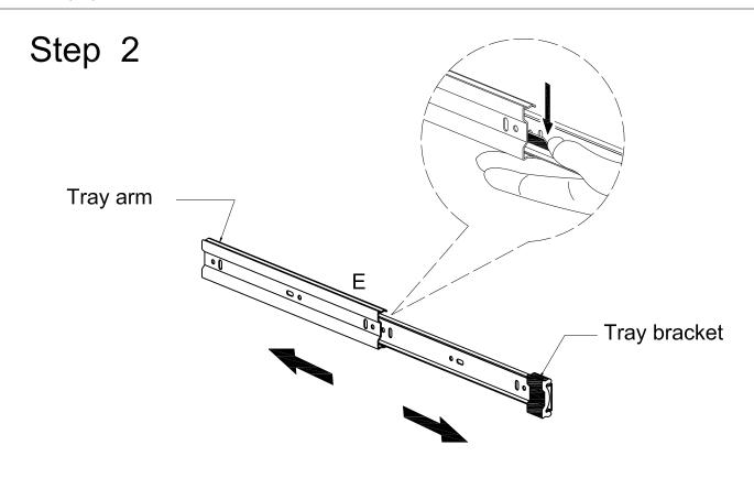
Disassemble keyboard tray sliders (E): Slide the tray arm and tray bracket apart then depress the small lever on the tray bracket and carefully pull the two pieces apart.
