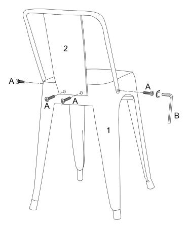
Assemble the back panel (2) to the chair (1) by using bolts (A) and wrench (B).
