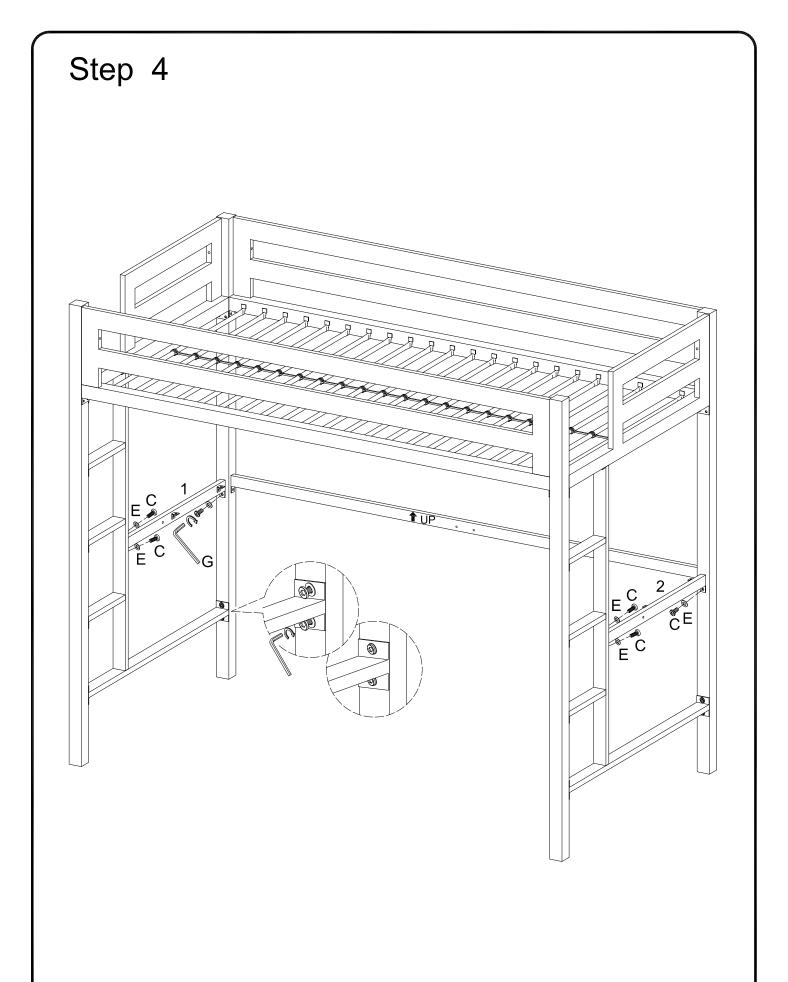
Attach crossbars (1,2) to the bunk bed frame using medium bolts (C) and washers (E). Retighten the bolts that secure the short crossbars.
