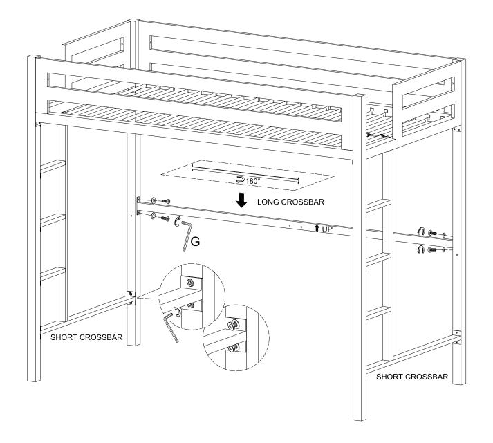
Remove the long crossbar from the bunk bed frame and turn it over so the screw holes are facing forward. Reattach the long crossbar to the bunk bed frame using the same bolts and washers from Step 1. Loosen, but do not remove the bolts that anchor the short crossbars to the bunk bed frame.
