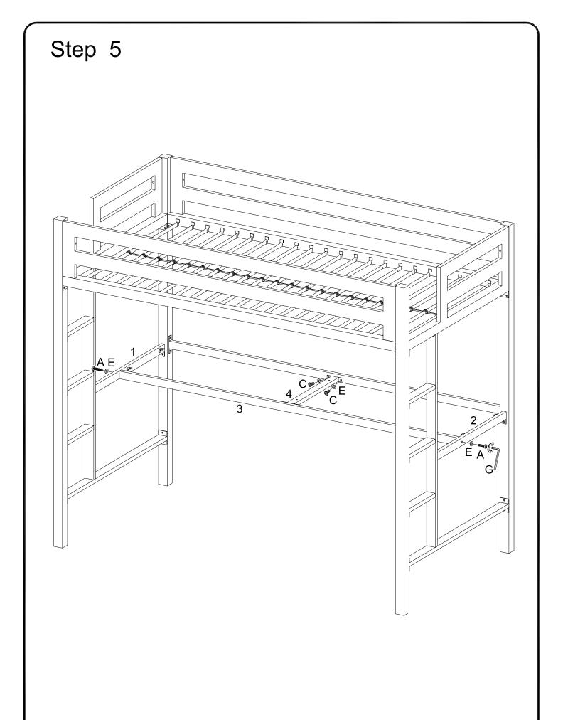
Attach crossbar (3) to crossbars (1,2) using bolts (A) and washers (E). Attach desk crossbar (4) to the bunk bed frame using bolts (C) and washers (E). Tighten all bolts with wrench (G).
