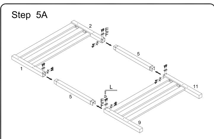
Assembly the three support posts by combining parts (1,5) and (9); then parts (2,5) and (11) as shown in the illustration. Secure these parts together using bolts (E) and washers (F). Be sure to tighten firmly using wrench (L).
