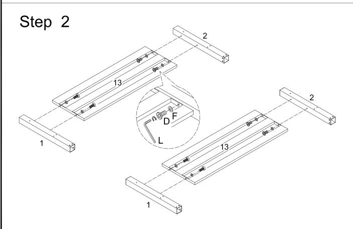
Secure guardrails (13) to the supports posts (1,2,) using bolts (D) and washers (F) as shown in the illustration. Be sure to tighten firmly using wrench (L).
