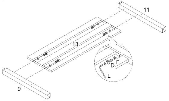
Secure guardrails (13) to the supports posts (9,11) using bolts (D) and washers (F) as shown in the illustration. Be sure to tighten firmly using wrench (L).
