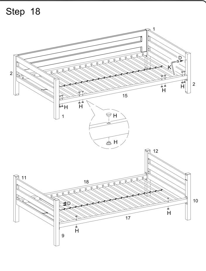
Place plastic plugs (H) into the holes in the front cross bars as shown in the illustration. Insert bolts (D) to support (2,9) using wrench (L).
