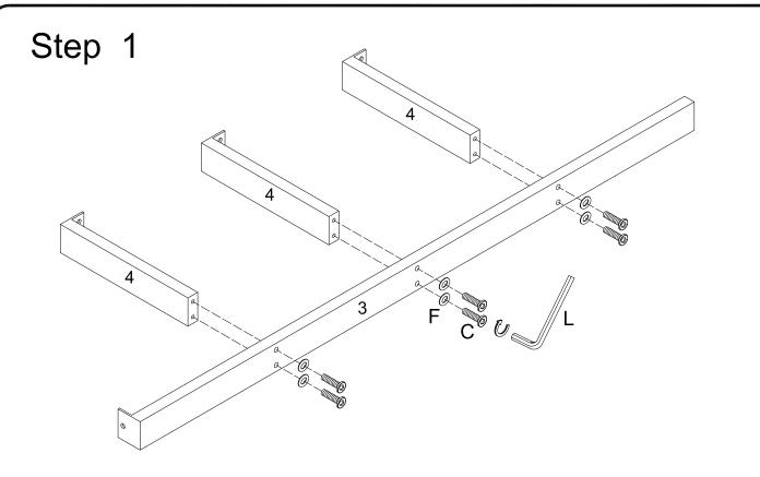
Attach the ladder steps (4) to the ladder support posts (3) using bolts (C) and washers (F) as shown in the illustration.
