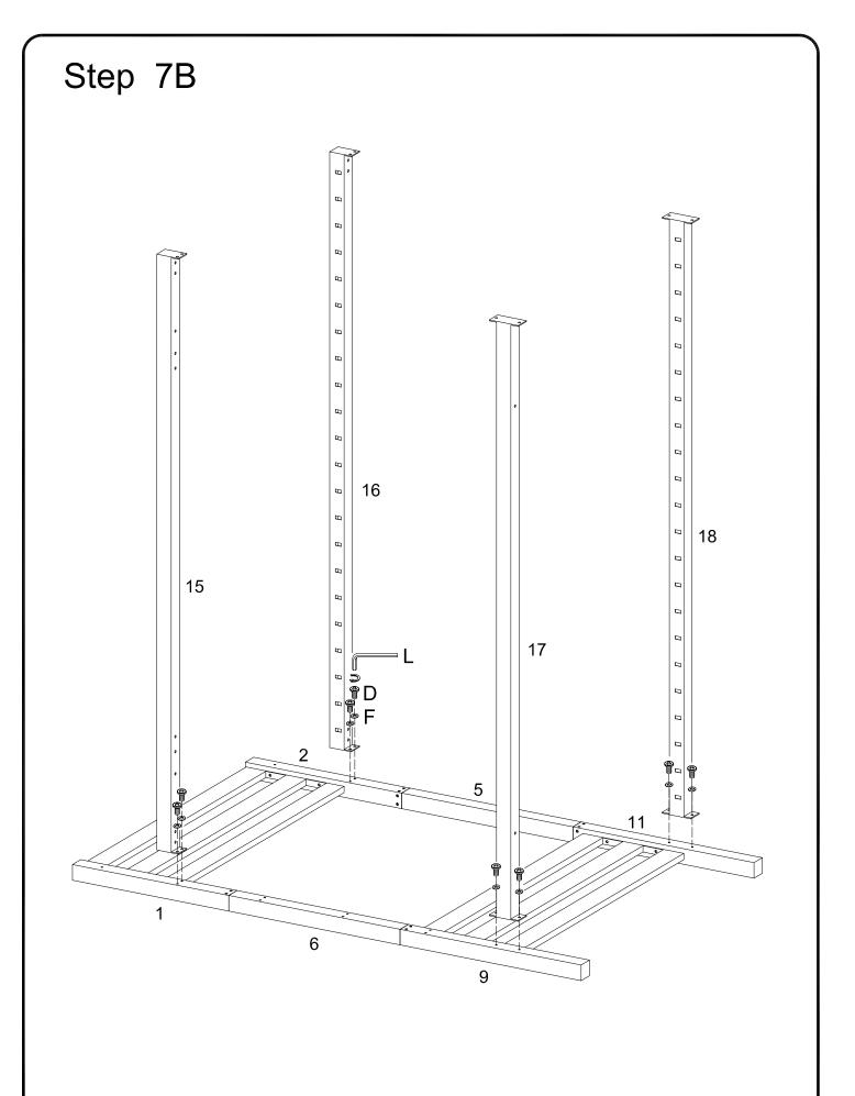
Attach lower cross bars (17,18) and upper cross bars (15,16) to the end supports in Step 5B using washers (F) and bolts (D) as shown in the illustration. Ensure the slots on the cross bats are facing inward as shown in the illustration. Be sure to tighten all bolts firmly using wrench (L).
