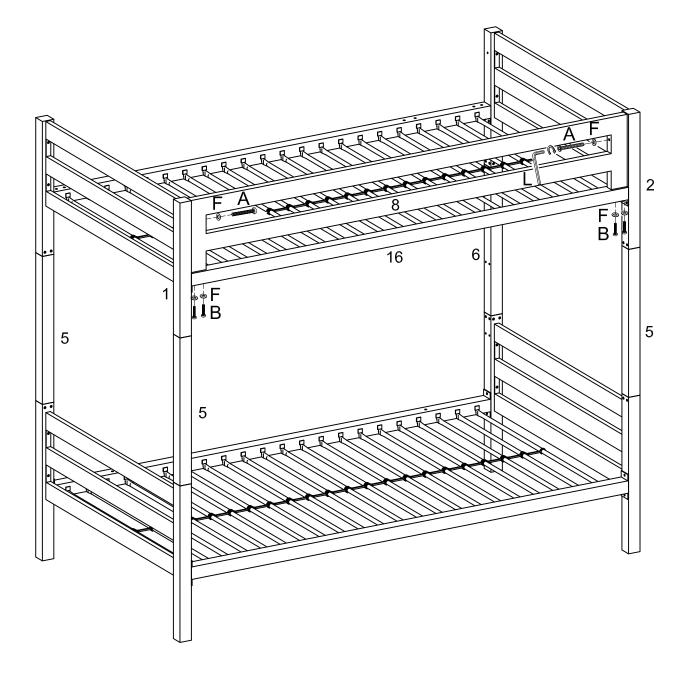
Attach back upper guardrail (8) to the back frame support beams using bolts (A) and washer (F) as shown in the illustration. Attach guardrail to cross bar (16) using bolts (B) and washers (F), tighten with wrench (L). Be sure to tighten all bolts firmly.
