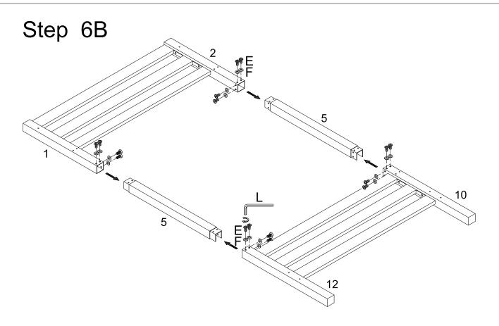
Assembly the three support posts by combining parts (1,5) and (12); then parts (2,5) and (10) as shown in the illustration. Secure these parts together using bolts (E) and washers (F). Be sure to tighten firmly using wrench (L).
