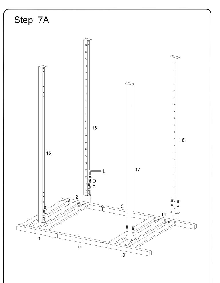
Attach lower cross bars (17,18) and upper cross bars (15,16) to the end supports in Step 5A using washers (F) and bolts (D) as shown in the illustration. Ensure the slots on the cross bats are facing inward as shown in the illustration. Be sure to tighten all bolts firmly using wrench (L).
