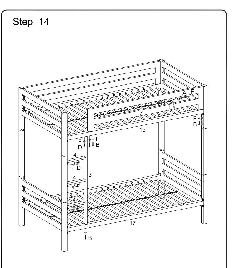
Loosen and remove the ladder support post (3), the ladder steps (4) and the open guardrail (7) from the bed frame.
