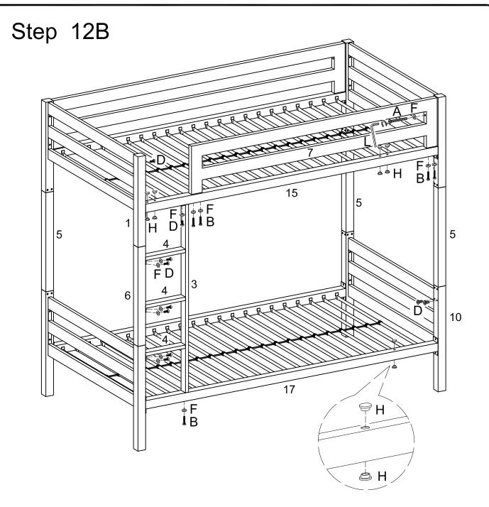
Attach ladder frame assembly to the upper cross bar on the right side using bolt (D) and washer (F) as shown in the illustration.
