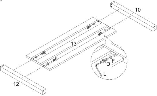
Secure guardrails (13) to the supports posts (10,12) using bolts (D) and washers (F) as shown in the illustration. Be sure to tighten firmly using wrench (L).
