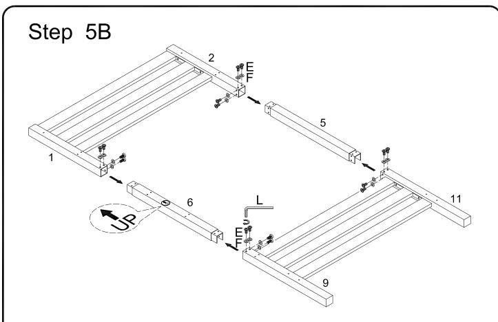
Assembly the three support posts by combining parts (1,6) and (9); then parts (2,5) and (11) as shown in the illustration. Secure these parts together using bolts (E) and washers (F). Be sure to tighten firmly using wrench (L).
