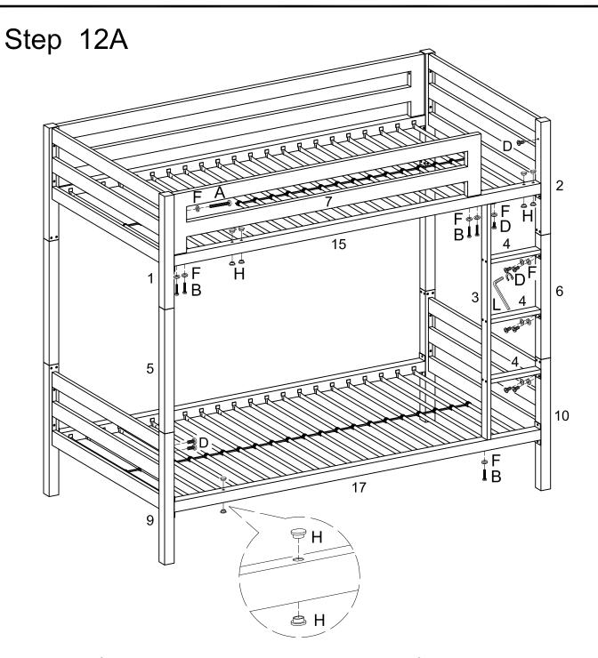
Attach ladder frame assembly to the upper cross bar on the left side using bolt (D) and washer (F) as shown in the illustration.
