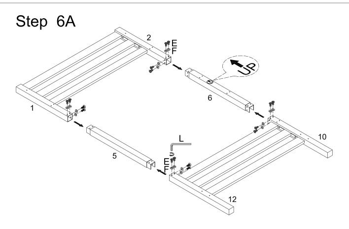
Assembly the three support posts by combining parts (1,5) and (12); then parts (2,6) and (10) as shown in the illustration. Secure these parts together using bolts (E) and washers (F). Be sure to tighten firmly using wrench (L).
